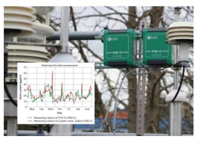
Outdoor measurement of the particulate in combination with other typical meteorological sensors. The RS485 signal can be connected to LSI-LASTEM data loggers (Alpha-Log, E-Log)
